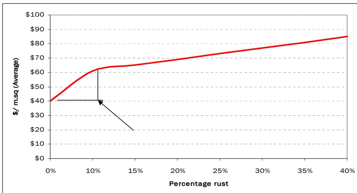
Graph 7 shows a number of Net Present Value (NPV) costs for a pylon located in a mild coastal environment.
