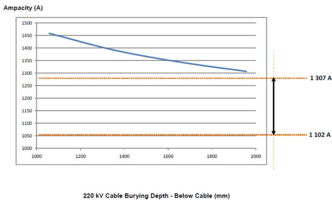
Figure 11: Effect of Increasing Burying Depth [3]
