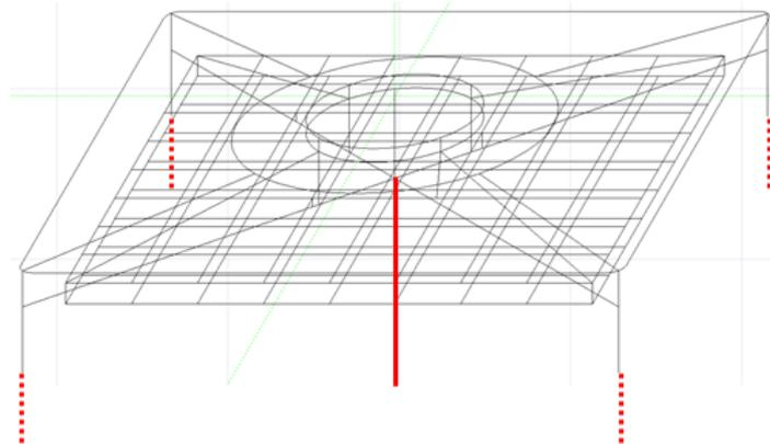
Figure 3: Variation to standard WTG earth grid design
