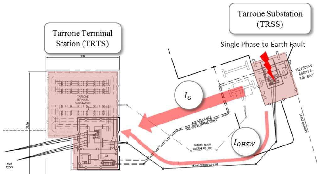
Figure 5: Fault current distribution – ground return & OHSW
