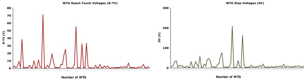
Figure 2: Result profiles of WTG earth grid
