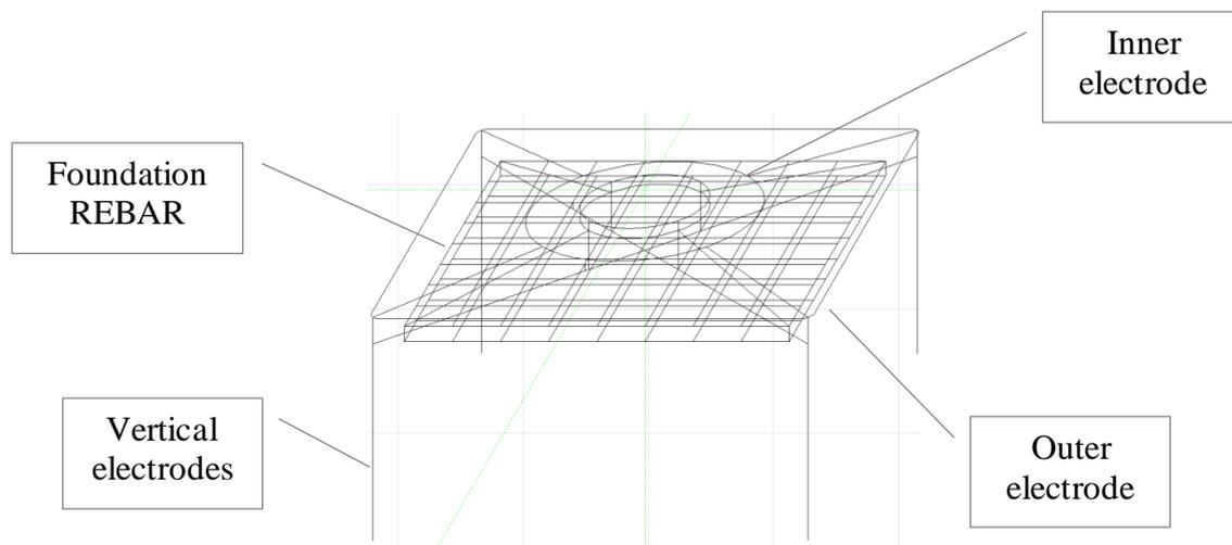
Figure 1: Basic WTG earth grid design
