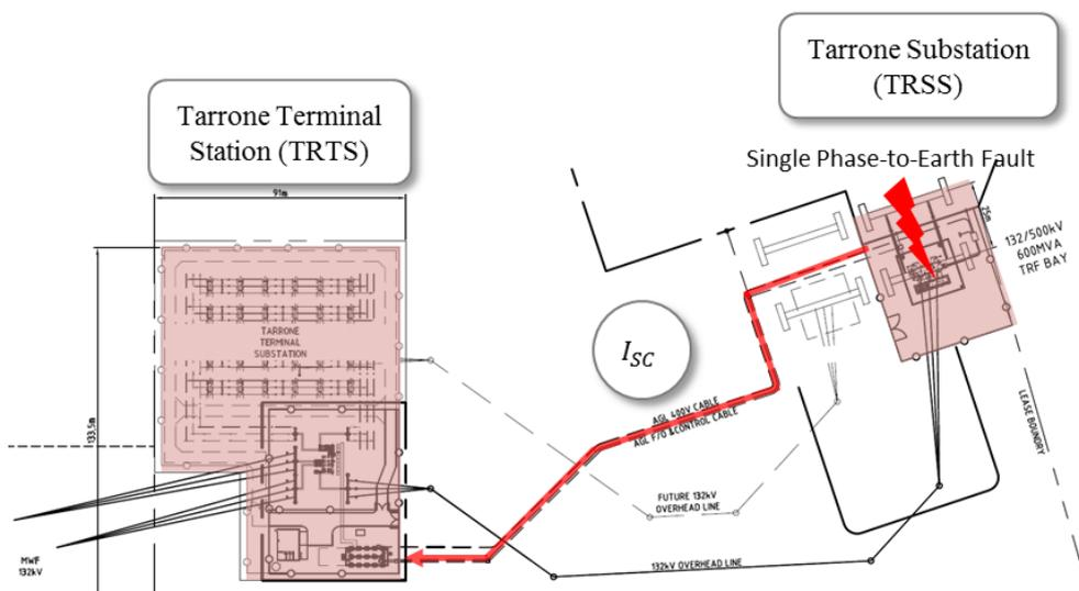
Figure 6: Fault current distribution – cable screens
