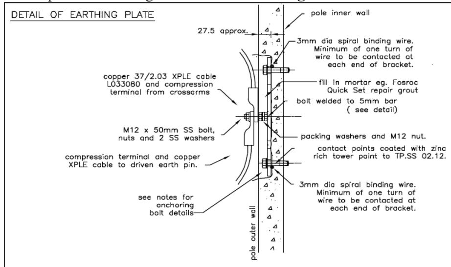
**Figure 2: Tentative Bonding Bracket Detail for Hollow Spun Poles.**
