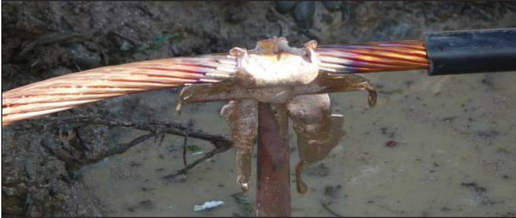
*Photo 5: Cadweld joint to earth-rod, showing excessive weld material leakage due to the taper at the top of the rod.*
