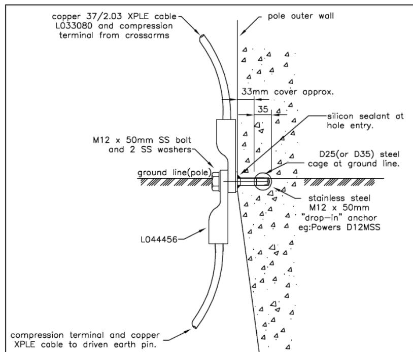
**Figure 1: Bonding details for Vierendeel poles.**
