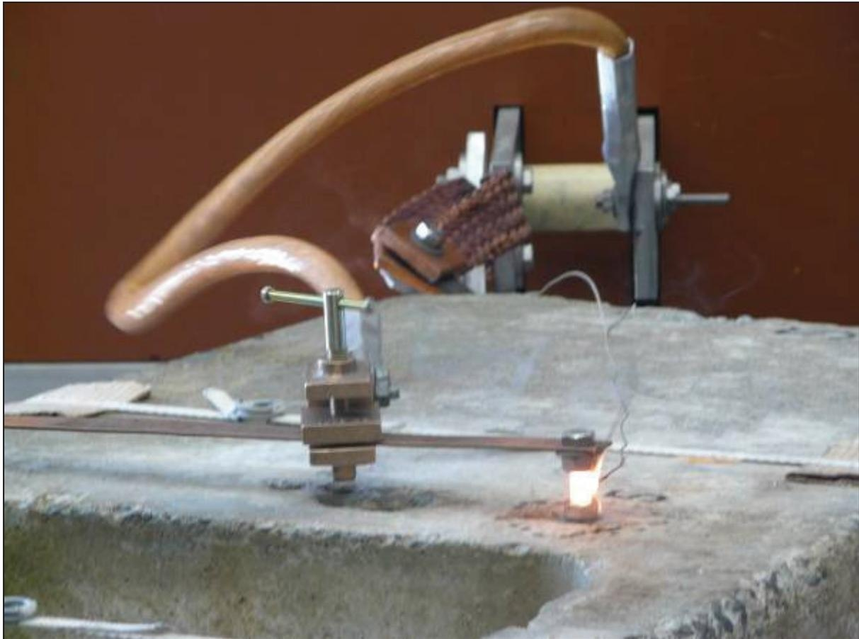
*Photo 1: High current testing Vierendeel pole cage bond, with connection bolt white hot.*
