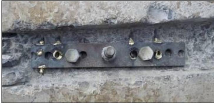
**Figure 9: Design 1B- Test sample 1- Brazed bonding plate joint.**
