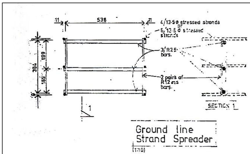
*Figure 2: Vierendeel pole ground line spreader cage*
