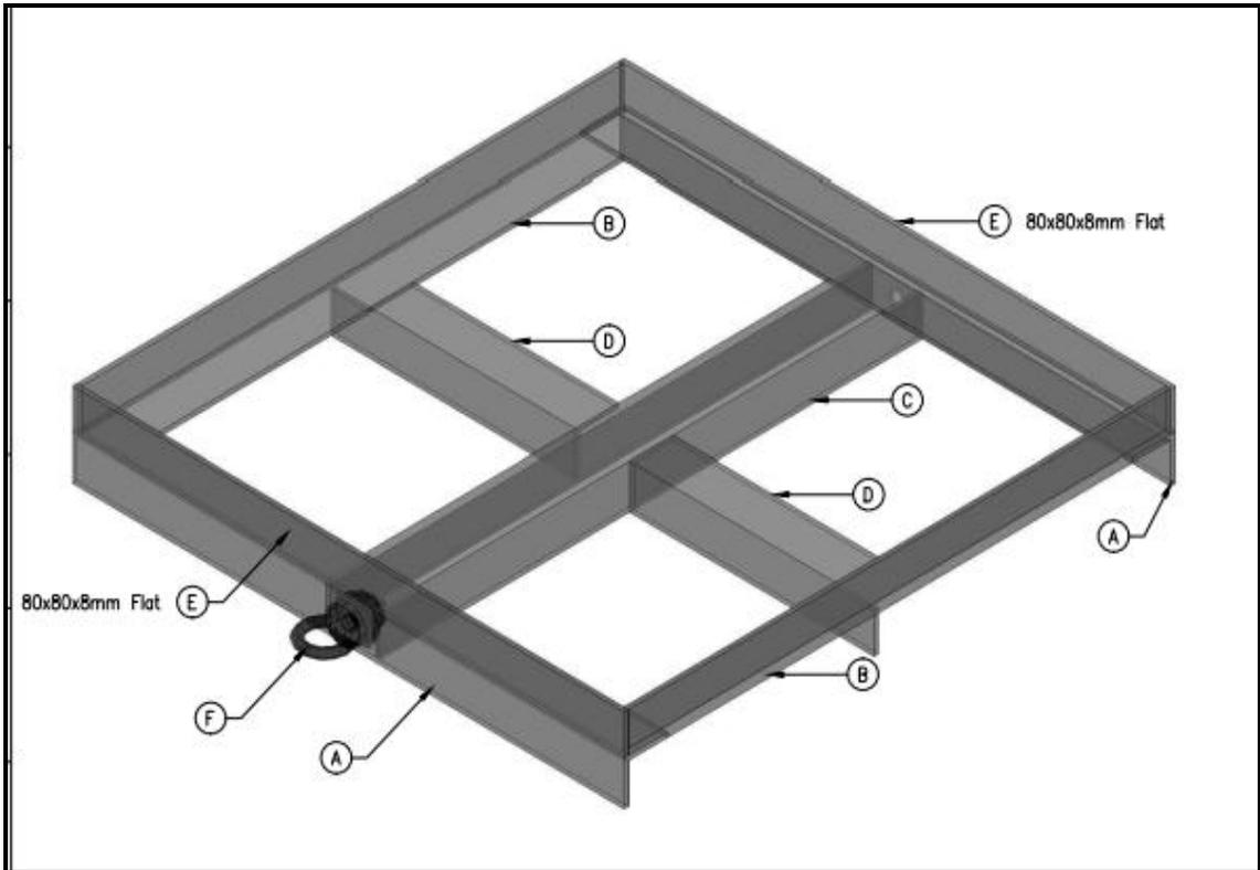
Figure 2: Surface Mount Stay Foundation Sled design
