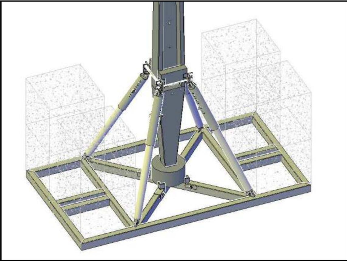
Figure 1: Surface Mount pole foundation design
