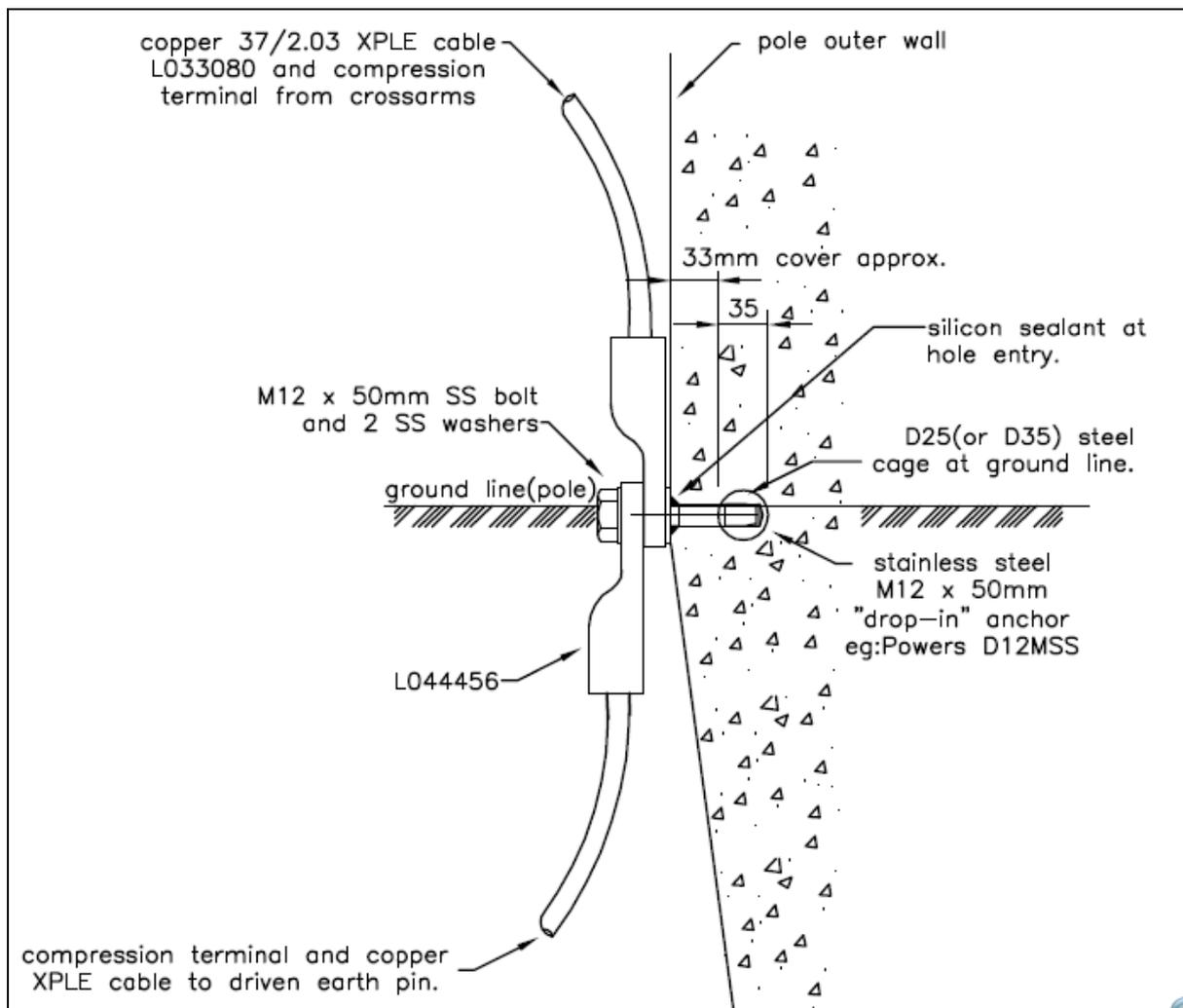
**Diagram 1: Tentative bonding bracket details for Vierendeel poles.**
