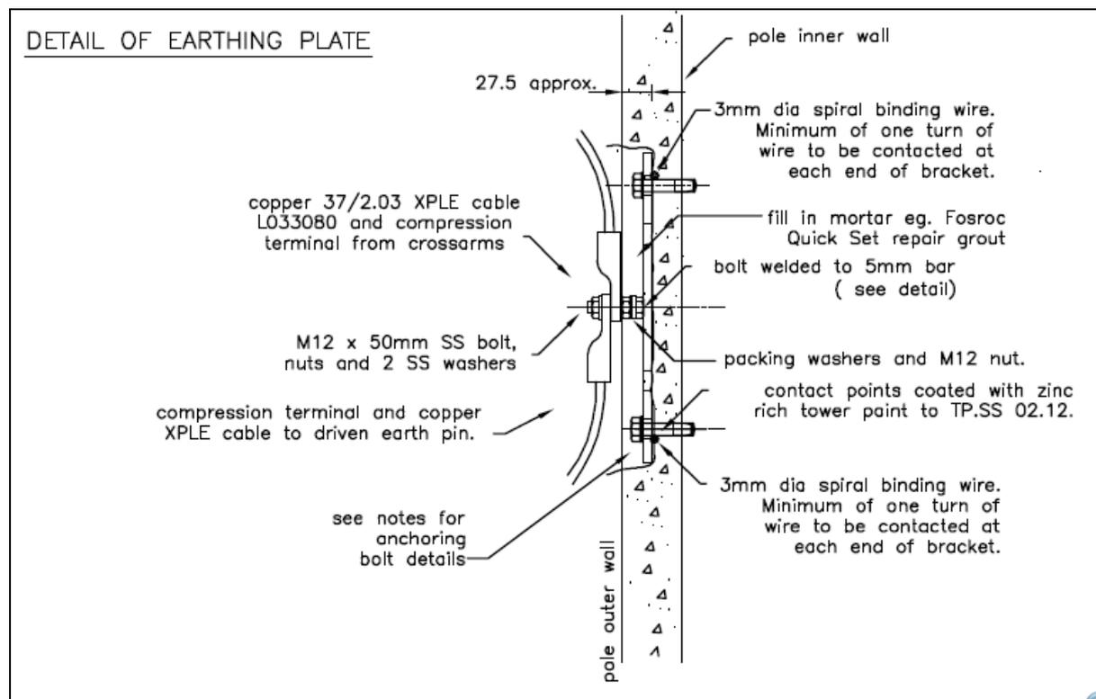
**Diagram 2: Tentative Bonding Bracket Detail for Hollow Spun Poles.**
