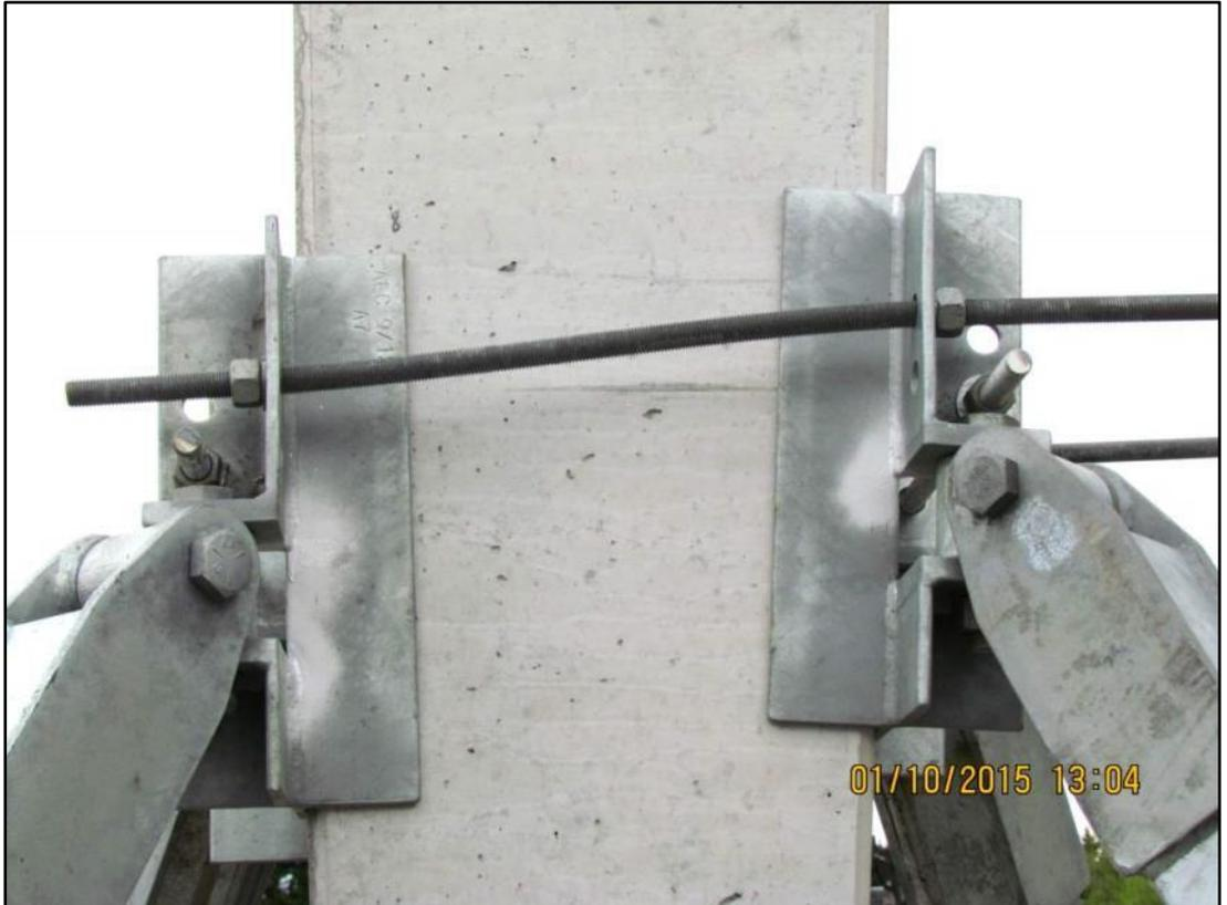
**Photo 6:** Heavy duty foundation upper clamping after test 2, showing differential vertical movement of clamps along the pole face.
