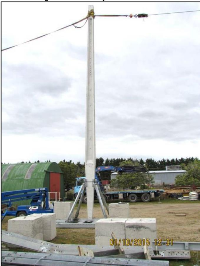
**Photo 4:** Heavy duty foundation under load test 1 (two diagonal blocks)
