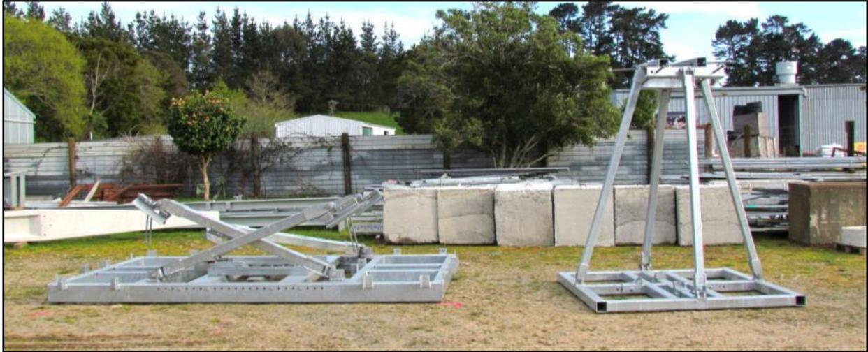
**Photo 1:** Heavy and light duty foundations side by side before testing. The concrete anchor blocks and test pole are in the background.
