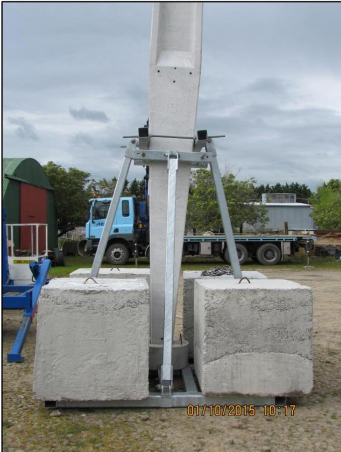
**Photo 3:** Light foundation pole lower section after test 4. Note the “S” bend in the clamping.
