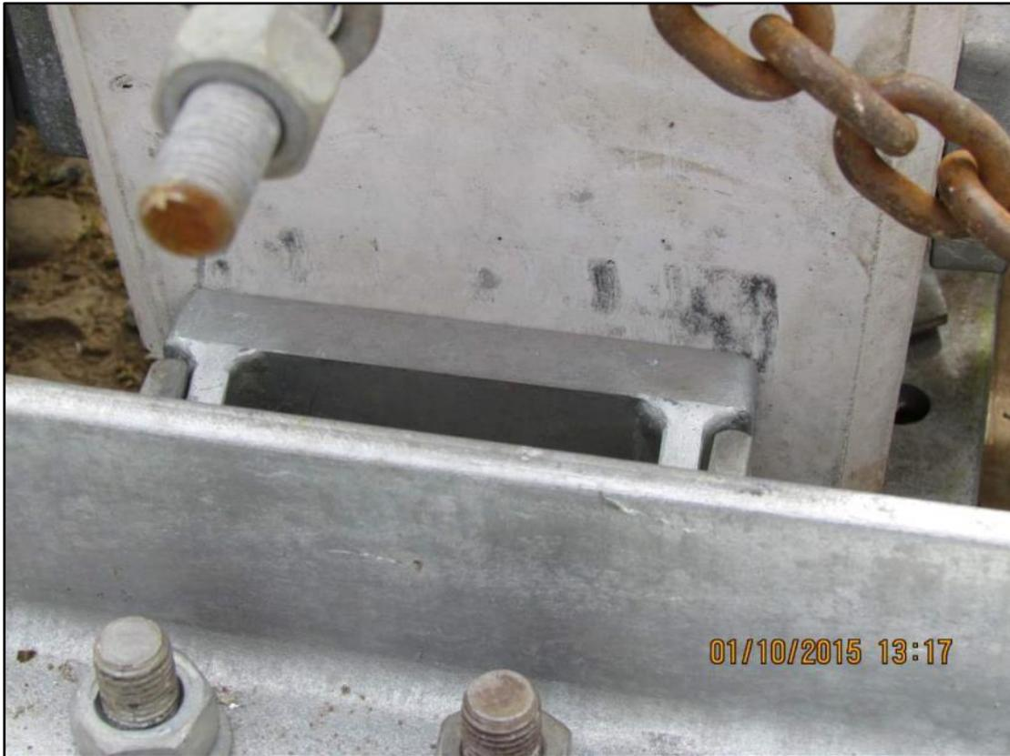
**Photo 5:** Heavy duty foundation butt clamping showing upward movement under test load 2
