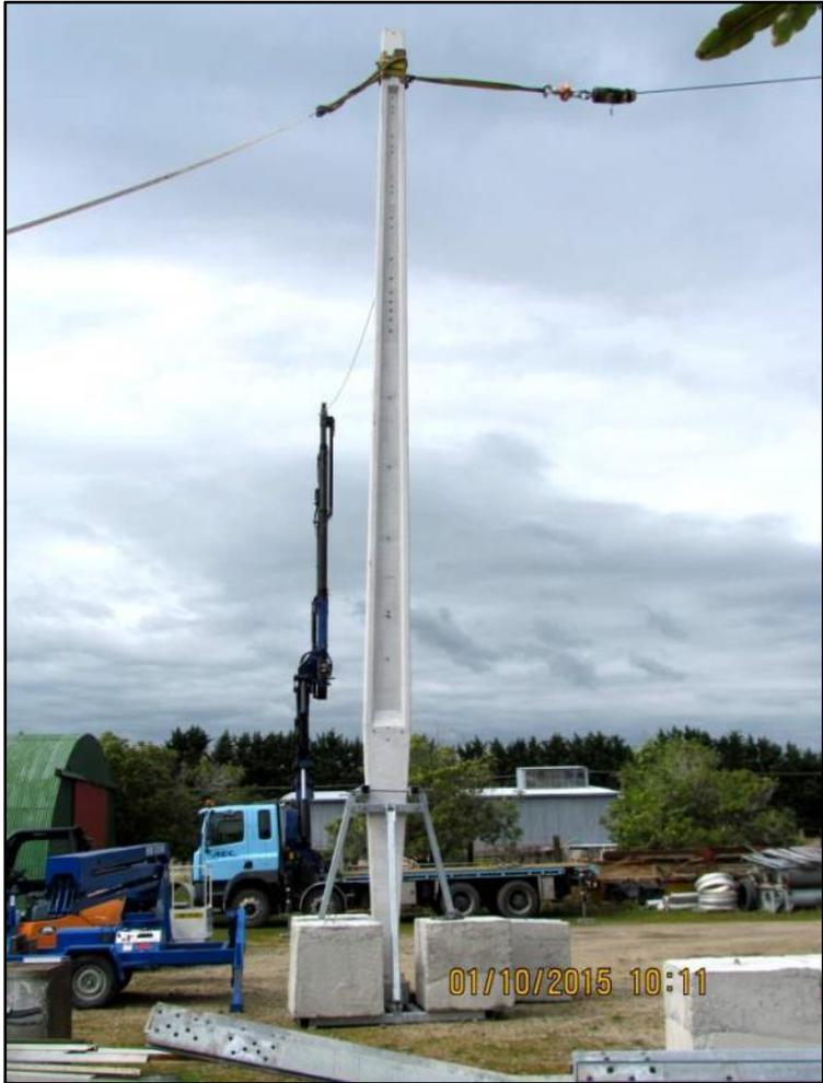
**Photo 2:** Light foundation under load test 3. (Three blocks)
